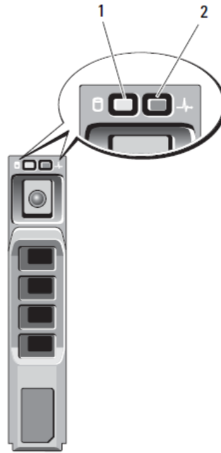
Figure 6. Hard Drive Indicators (includes HDD and SSD)
